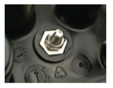
• Flash test valve: It is optional kits, made by plastic material.
