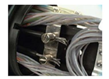
• **Grounding device:** A sealed grounding device can be pre-mounted in the base to connect metallic components to an external ground.
