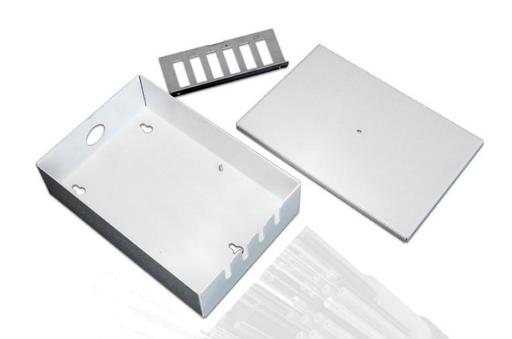
This tamperproof wall box terminates up to 24 fibres. It is a perfect cost-effective solution for FTTX networks. The adapter and connector meet on the inside of the wall box, ensuring complete security. It features 4 or 8 cable entry slots and 1 x 20mm cable entry gland hole.
