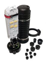
Our mechanical sealing dome closure is suitable for aerial, underground, wall mounting, manhole mounting and duct mounting applications. Made from injection moulded, high-strength engineering PC plastic, it is resistant to damage caused by extreme temperatures, oxygen and ultraviolet radiation. It features a compartment tray to store excess fibre.
